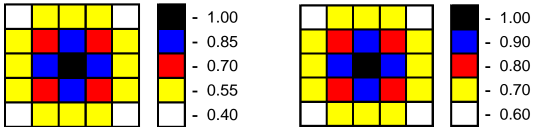
Figure 39. Subpixel average relative efficiency for Ortec (left) and PHDS DSSD (right).
